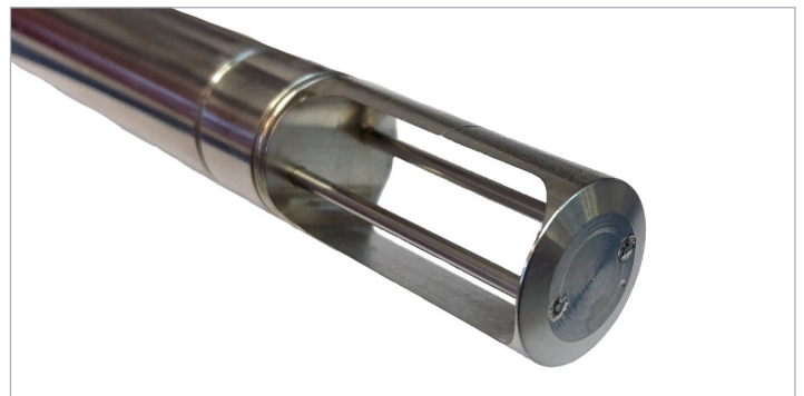
The Fox Thermal DDC-Sensor™ eliminates the sensor element vibration which can lead to metal fatigue and failure.
