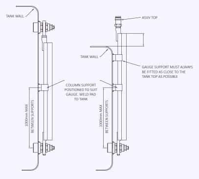
Gauges that have a centre distance greater that 1000mm and open circuit gauges, will be supplied with a column support, so that the gauge can be fixed to the tank wall. The maximum distance between the gauge fixings and a column support or between two column supports should be 1000mm, in the case of open circuit gauges the top most column support should be fitted as close to the tank top as possible.
