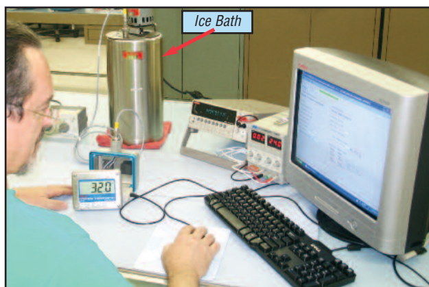
System Calibration of a Remote Digi-Stem utilizing an ice bath and DST/USB Interface Module.
