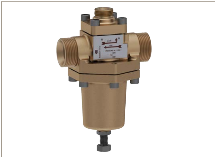
Parker Bestobell Cryogenic Pressure Regulator (Cryoreg) in Bronze (Inlet and outlet Ports 1-1/4" BSP-PL c/w 60° Cone; Economizer Port: 3/4" BSP-PL c/w 60° Cone)
