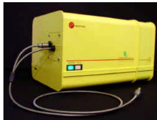
The PhytoScan system with a fiber optic bundle and a transreflectance probe.
